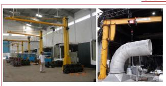
Available in different heights and capacities, Jib cranes are used for loading & unloading heavy machines, Material and high assembly work. These cranes consume less floor space and can be easily mounted on any existing structure.
